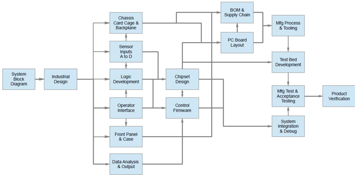
Figure 17: Network Diagram for Cardiac Monitor Development
